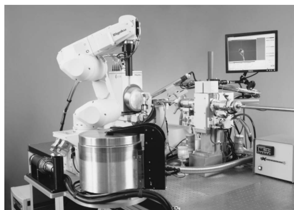
Fig. 2. An Example of a High Throughput X-ray Structure Analysis System
