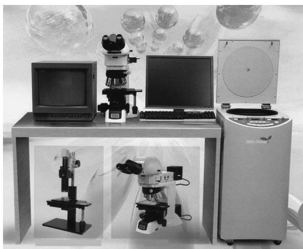
Fig. 6. Photograph of Apparatus for Measuring Adhesive Force by Centrifugal Separation Method
