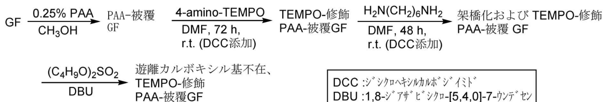
Fig. 1. Preparation Method of TEMPO-modified GF Electrode for Electroorganic Synthesis
