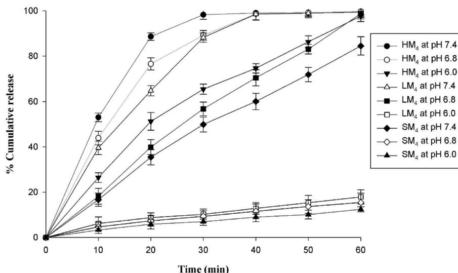
Fig. 2. Effect of pH on the Release of Enzyme from the Optimized Formulation of Papain Loaded Microspheres of HPMCP (HM<sub>4</sub>), Eudragit L 100 (LM<sub>4</sub>) and Eudragit S 100 (SM<sub>4</sub>) at pH 6.0, 6.8 and 7.4 Respectively
