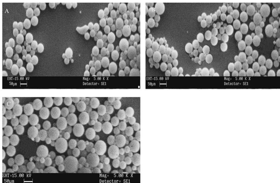
Fig. 6. SEM Photographs of Optimised Formulations of Papain Loaded HPMCP (A), Eudragit L 100 (B) and Eudragit S 100 Microspheres (C)
