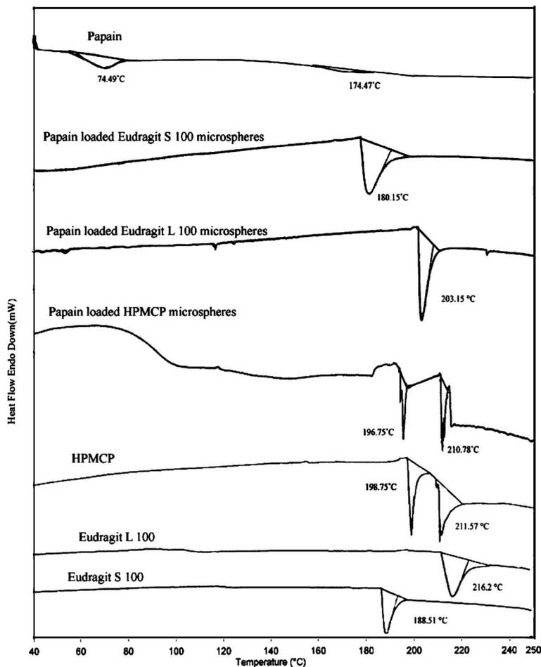
Fig. 5. The DSC Thermograms of Eudragit S 100, Eudragit L 100, HPMCP, Papain Powder and Optimised Formulations of Papain Loaded Eudragit S 100 (SM<sub>4</sub>), Eudragit L 100 (LM<sub>4</sub>) and HPMCP (HM<sub>4</sub>) Microspheres
