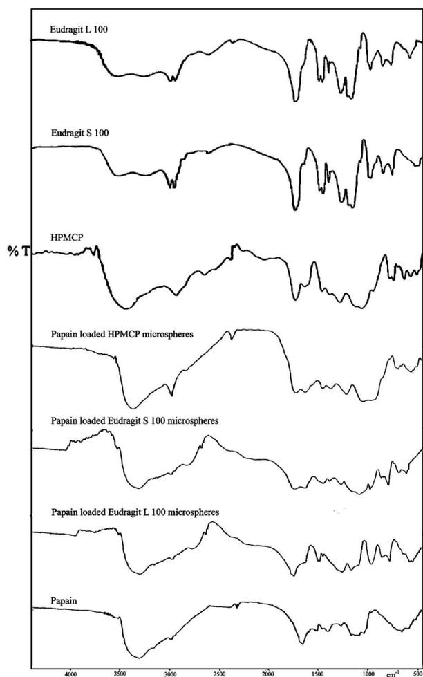
Fig. 3. The FTIR Spectra of Eudragit L 100, Eudragit S 100, HPMCP, Papain Powder and Optimised Formulation of Papain Loaded HPMCP (HM<sub>4</sub>), Eudragit L 100 (LM<sub>4</sub>) and Eudragit S 100 (SM<sub>4</sub>) Microspheres
