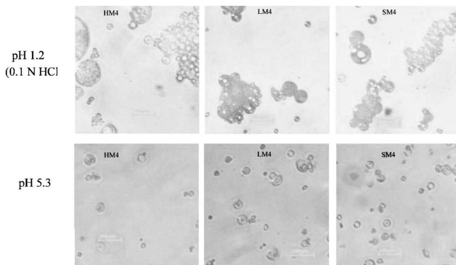
Fig. 1. Effect of Change in pH from pH 1.2 to 5.3 on the Aggregation and Deaggregation of Optimised Papain Loaded Enteric Microspheres of HPMCP (HM<sub>4</sub>), Eudragit L 100 (LM<sub>4</sub>) and Eudragit S 100 (SM<sub>4</sub>)
