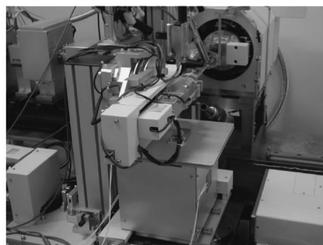
Fig. 1. Sample Mount Robot, SPACE
